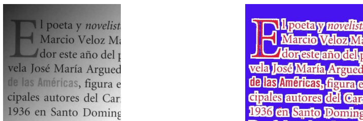
Original image and ternary local segmentation (white: background, red: object, blue: unknown)
