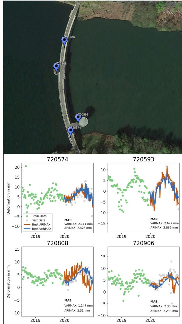
**Fig. 2.** Location of all PS points in ascending direction on the Lister Dam (top) and their corresponding deformation predictions for 2020 (bottom). For comparison, the best individual ARIMAX and VARMAX models are shown.
