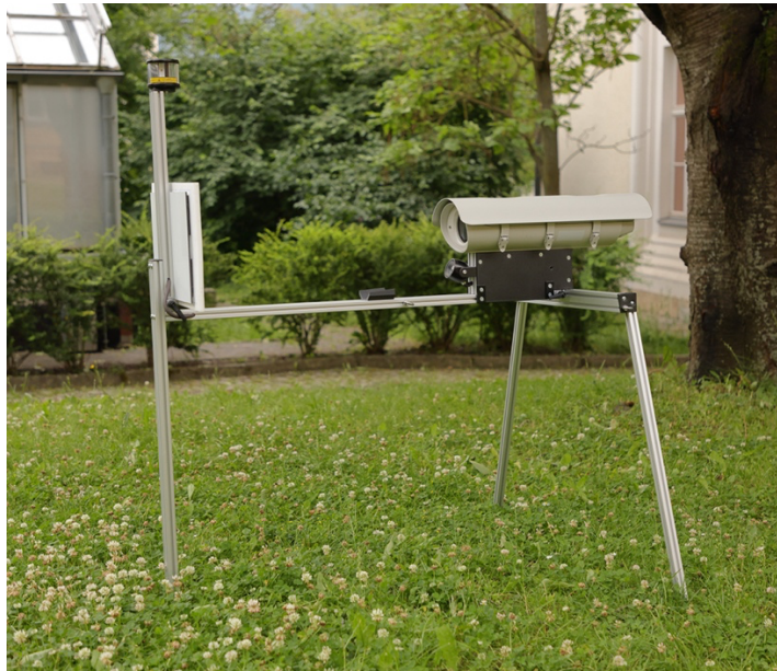
Fig. 8. Prototype of the new CLT design in the LEPMON project (August 2024). Instead of a DSL camera, an industrial camera along with electronic parts are accommodated in a waterproof housing.
