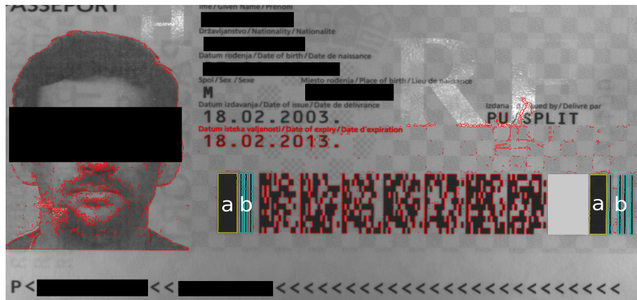
Fig. 2. Finding the barcode symbol by contour analysis. Elements of start and stop pattern marked, wide (a) and thin (b) rectangles.
