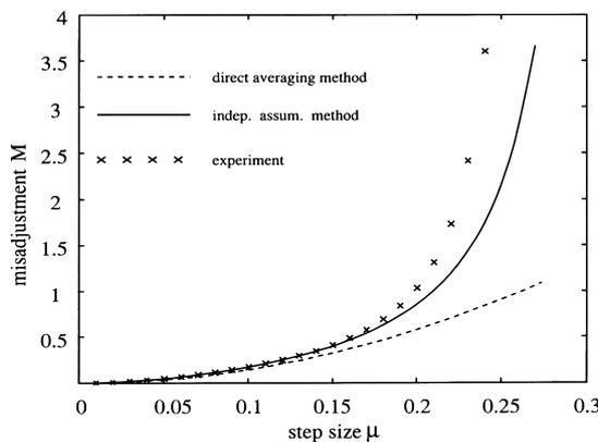
**Fig. 4** Comparison of the experimental results with the theoretical values for the misadjustment of the 2-D LMS in the simplified setting ( $\lambda_0 = \lambda_1 = \dots = \lambda_{N^2-1} = \sigma_x^2$ ,  $f_h = f_v = 0.5$ , and  $\mu_h = \mu_v = \mu$ ).
