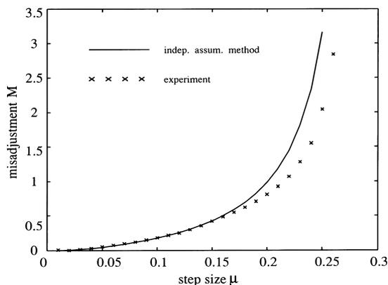
**Fig. 5** Comparison of the experimental results with the theoretical values for the misadjustment of the 2-D LMS in the simplified setting ( $\lambda_0 = \lambda_1 = \dots = \lambda_{N^2-1} = \sigma_x^2$ ,  $f_h = f_v = 0.5$ , and  $\mu_h = \mu_v = \mu$ ), i.i.d. binary input.
