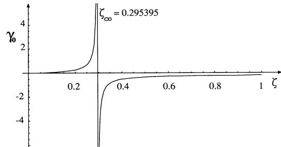
Fig. 2 Weight-error covariance coefficient  $\gamma_0$  as a function of  $\zeta = \mu\sigma_x^2$  for 2 by 2 adaptive FIR filter.
