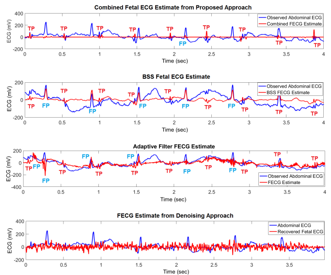
Fig. 20. Top to Bottom: Performance comparison of the proposed technique with the BSS, Adaptive filtering, and Denoising approaches, respectively using real dataset 2 (Blue: Abdominal ECG, Red: Estimated fetal ECG). TP marks a 'True Positive' event, FP a 'False Positive' event, while FN marks a 'False Negative' event. Note that a TP event is marked around 3.5 seconds because of detection of a FECG pulse that was overlapped by a MEGC pulse in the abdominal recording
