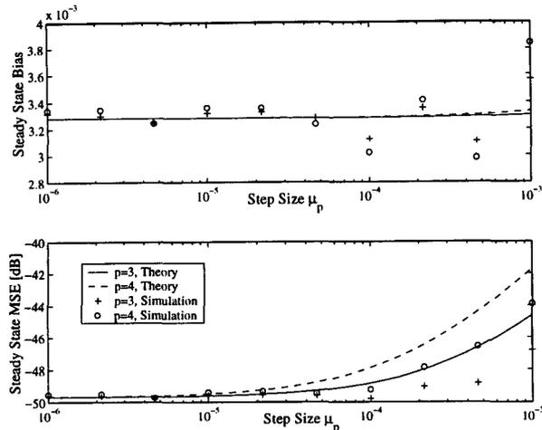
Figure 3: Comparison between theoretical and simulated steady state bias and MSE versus the step size value  $\mu_p$  ( $\rho = 0.9$ ,  $\omega_0 = 0.3\pi$ ,  $A = \sqrt{2}$ ,  $\text{SNR}=5$ ).
