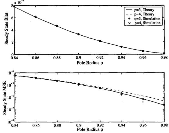
Figure 2: Comparison between theoretical and simulated steady state bias and MSE versus the pole radius  $\rho$  ( $\mu_p = 0.00005$ ,  $\omega_0 = 0.3\pi$ ,  $A = \sqrt{2}$ ,  $\text{SNR}=5$ ).
