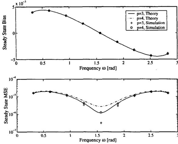
Figure 1: Comparison between theoretical and simulated steady state estimation bias and MSE versus the sinusoidal frequency of the input signal  $\omega_0$  ( $\mu_p = 0.00005$ ,  $\rho = 0.9$ ,  $A = \sqrt{2}$ ,  $\text{SNR}=5$ ).
