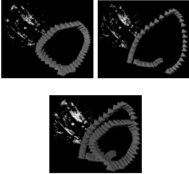
Fig. 3 Example for the registration of image sequences. Top Row: Calibration of two image sequence showing the camera positions as pyramids and 3-D point clouds in the background. Bottom: Registration of the two image sequences.
