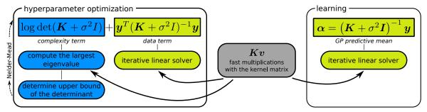
Fig. 2 Main outline of our approach for GP classification and hyperparameter optimization using fast multiplications with the kernel matrix. Details are given in Sect. 5 and Sect. 6.
