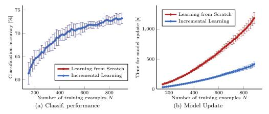
Fig. 11 Comparison of incremental learning and learning from scratch: (a) classification results achieved by both methods (the graphs are identical), (b) corresponding times for retraining the classifier when new data is accessible.
