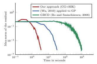
Fig. 6 Evaluation of the runtime and convergence of linear solvers: (1) our conjugate gradients method, (2) the coordinate descent method of Wu (2010), and (3) greedy block coordinate descent of Bo and Sminchisescu (2012).
