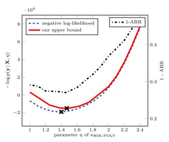
Fig. 12 Comparison between our upper bound of the negative marginal log-likelihood, the real negative marginal log-likelihood (left y-axis), and resulting ARR on the test set (right y-axis). Different hyperparameter values for HIK-POLY are shown on the x-axis.
