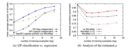
Figure 5.8: (a) Comparison of GP regression and classification (probit model, Laplace approximation) for independent and transfer learning. (b) Analysis of the average value of the task correlation parameter  $\rho$  with respect to the number of training examples (DepGP-Reg).
