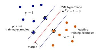
Figure 2.4: Basic principle of margin maximization with support vector machines. Colored points represent training examples and are additionally highlighted if they are support vectors.
