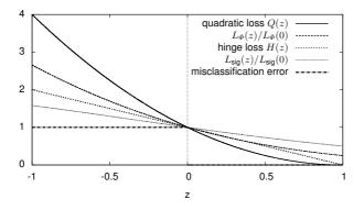
Figure 2.7: Visualization of different loss functions: hinge loss used by SVM, quadratic loss used by GP regression,  $L_{\Phi}$  and  $L_{sig}$  utilized for GP classification. These loss functions are compared to the misclassification error function shown in black color. This figure is best viewed in color.
