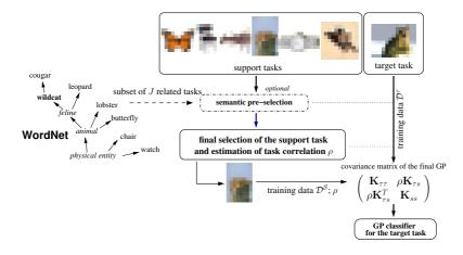
Figure 3.4: Basic outline of the proposed transfer learning approach: Semantic similarities between categories and leave-one-out estimates are utilized to select a support task, which is used to transfer knowledge to a target task with dependent Gaussian processes.
