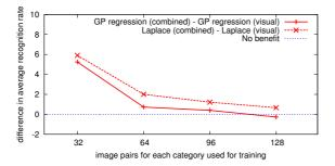
Figure 5.30: Performance benefit when using multiple sensors: Especially, learning with few examples benefits from multiple sensors. For GP regression the information present in 128 color training images seems to be sufficient, such that the noisy range images of the ToF camera do not help to improve the recognition performance anymore.
