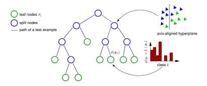
Figure 2.2: General principle and terms of decision trees. The right diagram illustrates the posterior distribution corresponding to a leaf node. The path of an example in the tree (dashed line) is determined by base classifiers related to each split node.
