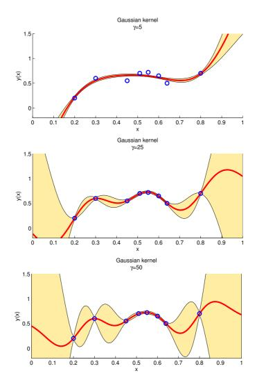
Figure 2.6: Examples of Gaussian process regression with the Gaussian kernel (2.41) and a varying kernel hyperparameter  $\gamma$ . The red graph displays the predictive mean function (2.77) and the shaded area highlights the interval derived from three times the posterior standard deviation. The standard deviation of the noise was set to 0.01.
