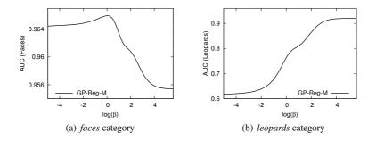
Figure 5.16: Influence of an additional smoothness parameter  $\beta$  of a modified image kernel function on the OCC performance for the object categories *faces* and *leopards*.
