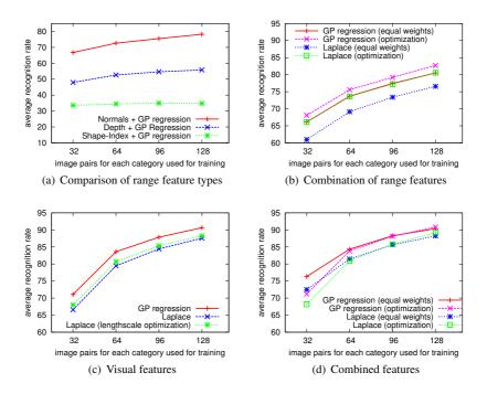
Figure 5.29: Evaluation of (a) different types of range features; (b) GP methods with multiple range features; (c) GP methods with color features; (d) and combined features from the CCD camera and the ToF camera. 32 image pairs correspond to one object instance or type.
