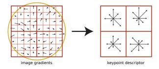
Figure 4.2: Calculation of the SIFT descriptor: (1) image gradients are calculated in a pixel neighborhood and weighted with an isotropic Gaussian mask; (2) an orientation histogram is computed for each block. Note that this visualization is simplified and uses a  $8 \times 8$  rather than a  $16 \times 16$  sample array (Lowe, 2004).
