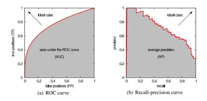
Figure 5.1: Performance measures for binary classification: (a) receiver operator characteristic (ROC) curves with the area under the ROC curve (AUC) criterion shown as a shaded area; (b) precision-recall curves with the average precision shown as a shaded area.
