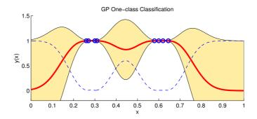
Figure 3.9: GP regression using a zero-mean GP prior in a one-dimensional OCC setting. The predictive distribution is visualized with its mean (red graph) and the corresponding confidence interval derived from the posterior variance. Training points are marked as circles. The dashed line shows the predictive variance as a function.
