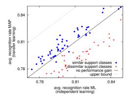
Figure 5.13: Average recognition rate of the ML approach in comparison to the rate after applying our MAP re-estimation technique. The regularization results in a performance gain only if support classes are (visually) similar to the target class.
