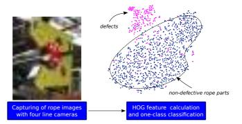
Figure 5.22: Rope images are captured by four line cameras arranged to analyze a wire rope (Moll, 2003). The scatter plot on the right hand side visualizes the high-dimensional histogram of oriented gradients features with the unsupervised *t*-SNE method of van der Maaten and Hinton (2008). Feature vectors are extracted from real rope data (ROPE1, view 3).
