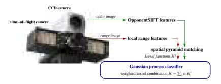
Figure 5.27: An overview of the proposed approach: color and range images are captured using a CCD camera and a time-of-flight camera (PMD Vision Technologies 19k); Local features are extracted from the data of both sensors and "kernelized" using spatial pyramid matching, which yields different kernel functions.
