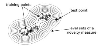
Figure 1.5: The principle of one-class classification and outlier detection: the distance of a test point to the training set is calculated with a novelty measure, which relates to the underlying data distribution.
