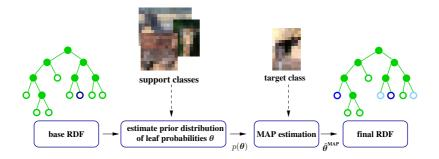
Figure 3.1: Outline of the regularized tree approach presented in Section 3.2: We build a random decision forest (RDF) using all training data, in which leaf probabilities of a target class are re-estimated using a prior distribution obtained from a set of support tasks. Shaded nodes in the decision tree are leaves with non-zero posterior probability of the target class.
