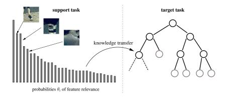
Figure 3.3: Illustration of the general principle of our approach: Feature relevance is estimated from a support task and used to regularize the feature selection in the training process (random decision forest) of a target task with few training examples. The probabilities and BoV feature visualizations are directly obtained from our image categorization task (Section 5.2).
