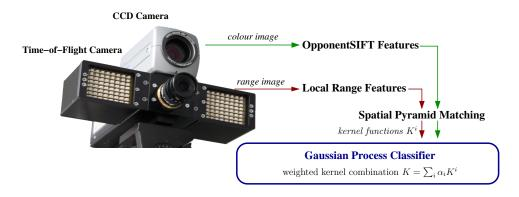
**Figure 1:** An overview of the proposed approach: colour and range images are captured using a CCD camera and a Time-of-Flight camera (PMD Vision Technologies 19k); Local features are extracted from the data of both sensors and "kernelized" using Spatial Pyramid Matching, yielding different kernel functions.
