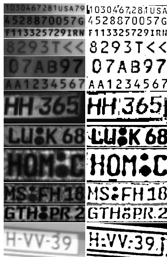
Figure 5. Examples for segmentation results within a license plate and id card recognition scenario: Black color corresponds to pixels marked as object pixel during our local segmentation step. Segmentation artefacts can be easily filtered in an additional post-processing.
