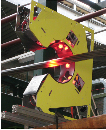
Figure 2: A prototype version of the device which acquires the rope data
