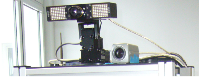
Fig. 1. Setup of our place recognition system with a ToF sensor and a visual sensor mounted on a mobile robot. Data is obtained from both uncalibrated cameras in order to build the combined feature representation of the current view.
