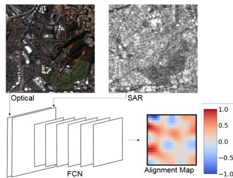
**Fig. 1:** Scheme of the proposed deep metric. The concatenated input of the FCN consists of a fixed optical image and a SAR image which is transformed during registration. The scalar deep metric value is calculated by the averaging of the spatially-resolved output of the FCN that predicts the alignment of its input channels.
