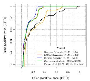
**Figure 3:** *ROC curves of the presented VAR-based defect detection model for various dependency analysis methods. The results of the model from [PNWD09] are included for a comparison. The experiments were performed on a real wire rope data set.*
