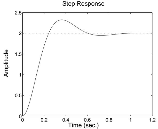
Fig. 1. Step response of a second order system
