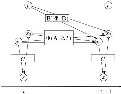
Fig. 2. Weight matrices in a Kalman filter
