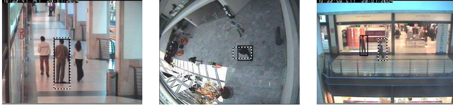
Figure 2. Stills from three of the videos used. The solid box marks the hand-labeled ground truth. The dashed box is the tracker’s current estimate. In the right-most image, the tracker has been distracted by a temporary occlusion from another person, and subsequently lost the real target.
