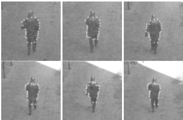
Figure 8: Sequence 1: Tracking a pedestrian with active rays. (images 4, 24, 44, 64, 84, 104 of a sequence taken during a real-time experiment). The sampling step size \Delta\phi is 2\pi/15 .
