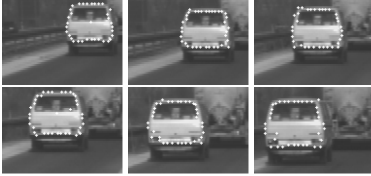
Figure 9: Results for tracking a car on a highway with active rays (images 4, 24, 44, 64, 84, 104 of a sequence of 123 images taken at video rate): the sampling step size \Delta\phi is \pi/18 .
