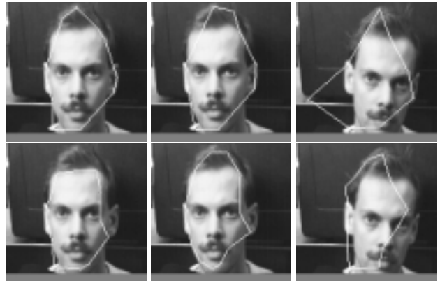
Figure 5: Results of the offline tracking with DP (first row) and GRDY (second row) for the head-sequence.
