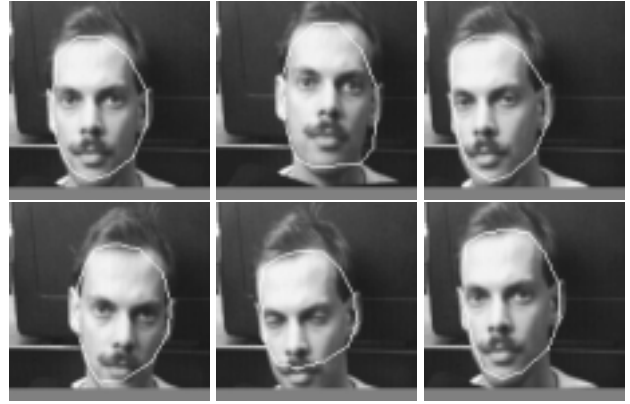
Figure 4: Results of the offline tracking with VARN for the head-sequence (images number 0,30,60,90,108,111). Images 108 and 111 show the effect of the blowing forces: Although partially losing the contour, the active contour catches again the contour of the head.
