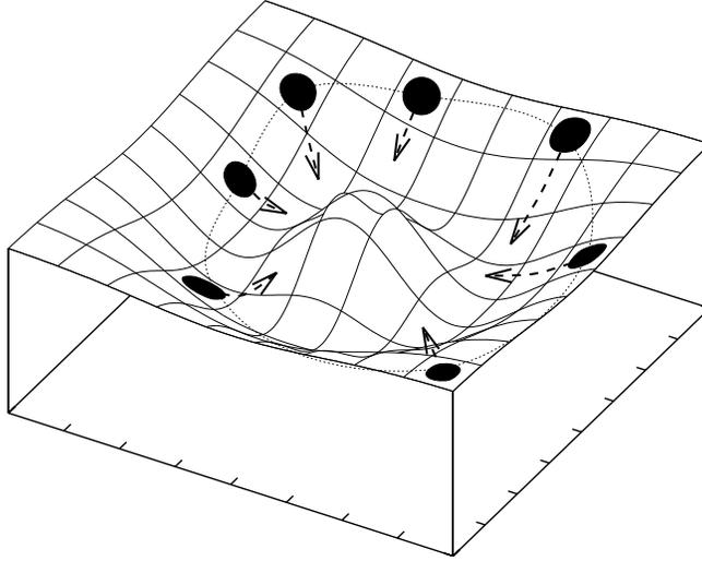
Figure 1: Principle of active contours: A snake with 7 elements extracts the contour of a circle by moving into the minimum of the negative edge strength of the circle.
