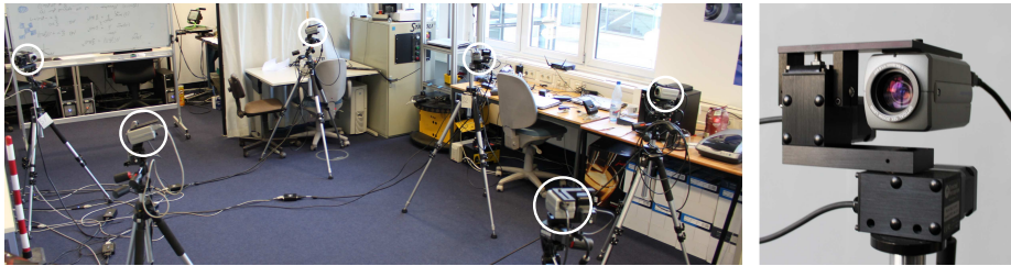
Fig. 1. A multi-camera system (left) consisting of six pan-tilt zoom cameras (white circles). The cameras are mounted near the intersection of the pan and tilt axes (right).
