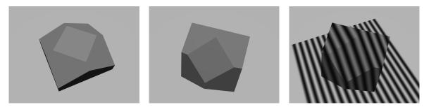
Figure 2. Example for lighting changes during a rotating prism around the x and z axis. Left the first image of the measurement sequence, the two other images are aquired at time step 21 - in the middle without any projection, right with a sinusoidal intensity distribution.
